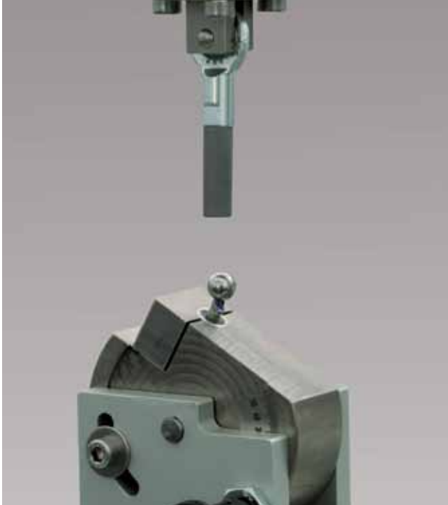
Swivelling test device for dental implants
