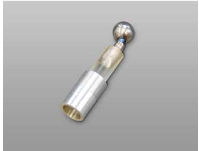
Dental implant which is embedded in a pot
